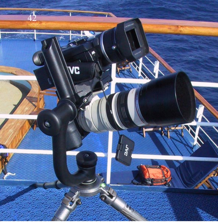
At left: My video and still cameras, piggybacked using a stock Wimberley Gimbal mount, on a Gitzo tripod. The combination is balanced and turns effortlessly.
